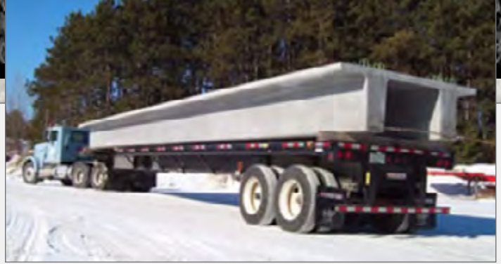
Example of one type of prefabricated bridge element
